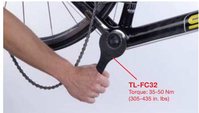
2. Use the special tool TL-FC32 to tighten. Right has a counter-clockwise thread. Left is clockwise. Use torque wrench to reach spec.
