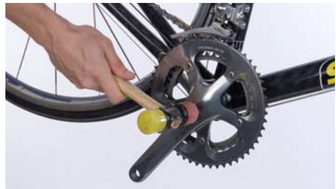
4. To make sure the crank is seated properly, tap over the center of the assembly with a rubber or plastic mallet.
