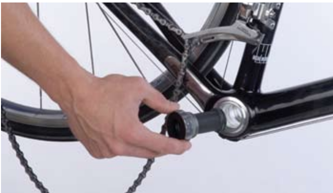
1. First install the right and left adapters.
